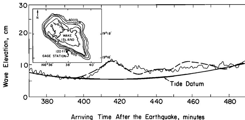
Fig. 1. The 1964 Alaskan tsunami observed at Wake Island by *Van Dorn* [1970] and compared with the prediction of the wave history by *Hwang et al.* [1972].
