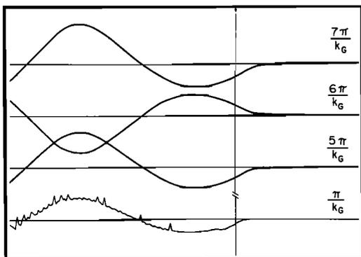
Fig. 2. Model tsunami wavelet formed by multiplying the Airy function by a Poisson distribution. See Figure 1.
